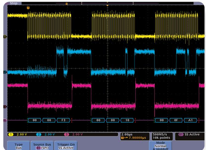
► **Figure 13.** Correct synthesizer configuration messages.
