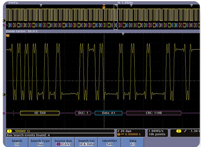
► **Figure 21.** Searching on specified Identifier and Data in a CAN bus acquisition.
